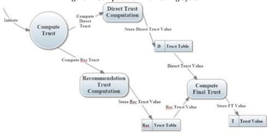
Figure 3: Trust Computation Process
