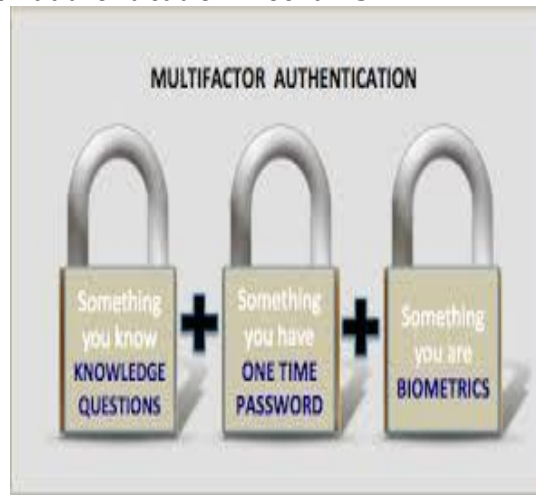
Figure 9: Design of Multi-factor authentication
