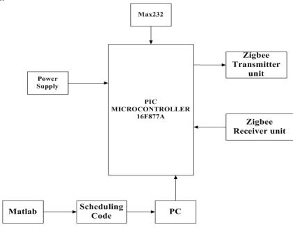
Figure 3.1: Base station Block Diagram
