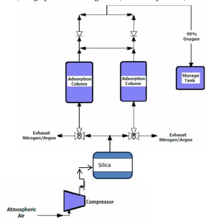
**Figure 9: PSA Process Flow Diagram**
