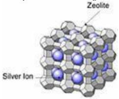
Figure 6: Zeolite A with Silver Ion
