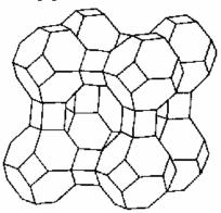
Figure 8: Zeolite a structure
