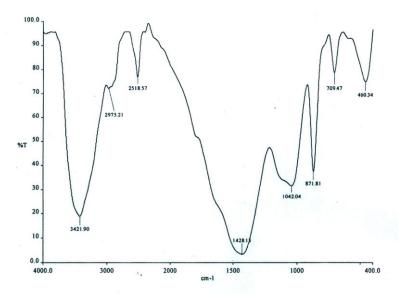
In the present work, the observed peak at around 800 cm<sup>-1</sup> is present in various spectra which may be assigned to Si-O bending vibrations. In almost all the samples, a peak at around 780 cm<sup>-1</sup> is present which may be assigned to Si-O-Si symmetrical stretching vibrations. The peak in the region 692–694 cm<sup>-1</sup> is a characteristic peak of quartz due to Si-O bending vibration. This peak is present all the samples. The sharp intense band at
